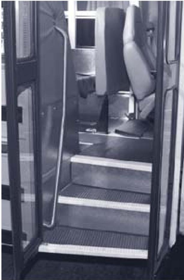
**Bus with three steps and low handrail**
