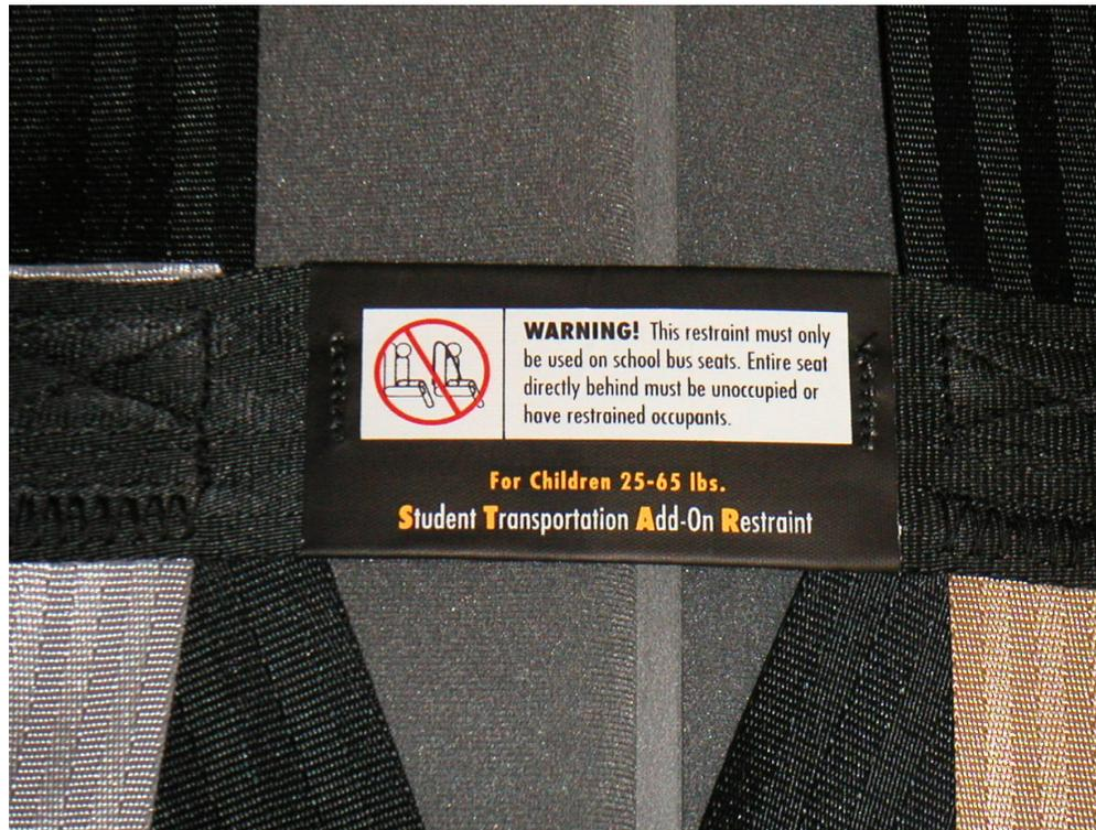
**WARNING!** This restraint must only be used on school bus seats. Entire seat behind must be unoccupied or have restrained occupants.
