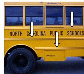
on body. Guardrails shall be installed utilizing Pan Head Carbon Steel Screws/stainless steel sheet metal screws/ or Drive rivets in all attaching positions
