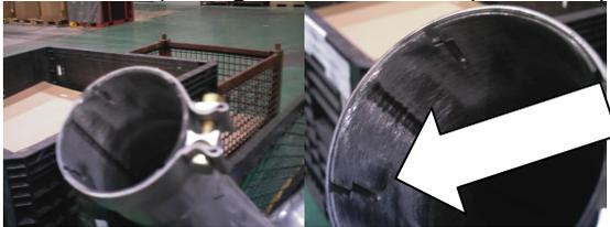
Arrow indicates offset collapsing slit.
