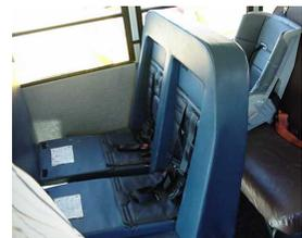
CSRS compliant seats shall be installed in the following standard locations.
