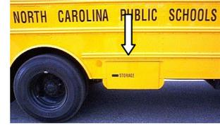
Warning Devices – Each school bus shall contain at least three reflective triangle road-warning devices that are enclosed in a storage box. These shall be mounted in the “Safety Equipment Storage Box” and must meet requirements in FMVSS 125.
