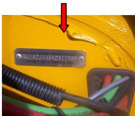
**SERIAL NUMBER LABEL** – A fireproof label shall be furnished showing the Vehicle Identification Number, and permanently affixed on the firewall in a position for maximum visibility and legibility (exact location to be approved). Letters and numerals shall be of the cut or embossed (metal) type. The serial letters and numerals should be at least one-fourth inch in height. (See picture for location).
