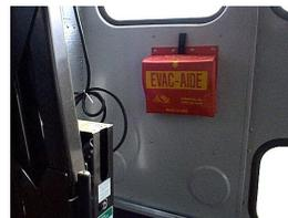
shall be attached to the interior wall in a manner that would retain the pouch to the wall when a 20G force is applied to the cabinet in any direction.
