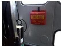
**Fire Blanket** - Each lift-equipped school bus shall be equipped with Tietech Model # 1007 fire blanket and shall be enclosed in a non-metallic pouch. It shall be identified on the front as to the contents. The pouch shall be mounted on the left side interior wall in the buffer zone, behind the left rear seat as close to the rear entrance door opening as practical on a horizontal and vertical line no higher than the horizontal metal portion of the seat frame.
