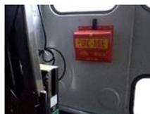
**Fire Blanket** - Each lift-equipped activity bus shall be equipped with Tietech Model # 1007 fire blanket and shall be enclosed in a non-metallic pouch. It shall be identified on the front as to the contents. The pouch shall be mounted on the left side interior wall in the buffer zone, behind the left rear seat as close to the rear entrance door opening as practical on a horizontal and vertical line no higher than the horizontal metal portion of the seat frame.
