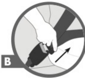
**B** CHECK that the buckle connection is secure by tugging firmly on the seat belt latch plate.
