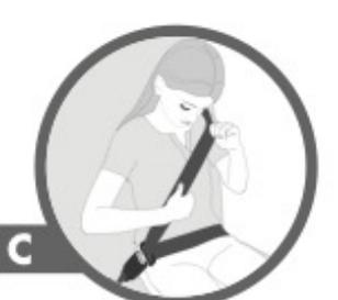
**C** TIGHTEN the lap portion by pulling upward on the shoulder belt. Be sure that the shoulder belt is snug across the chest and crosses the center of the shoulder.
