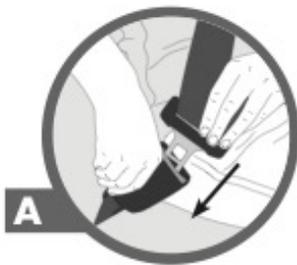
**A** BUCKLE the latch plate into the matching buckle after pulling out the shoulder belt webbing from the seatback. LISTEN for the CLICK sound when the latch plate is fastened!
