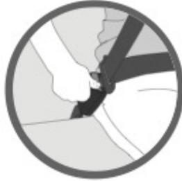
1. Push the red button on the buckle and remove the latch plate from the buckle.
