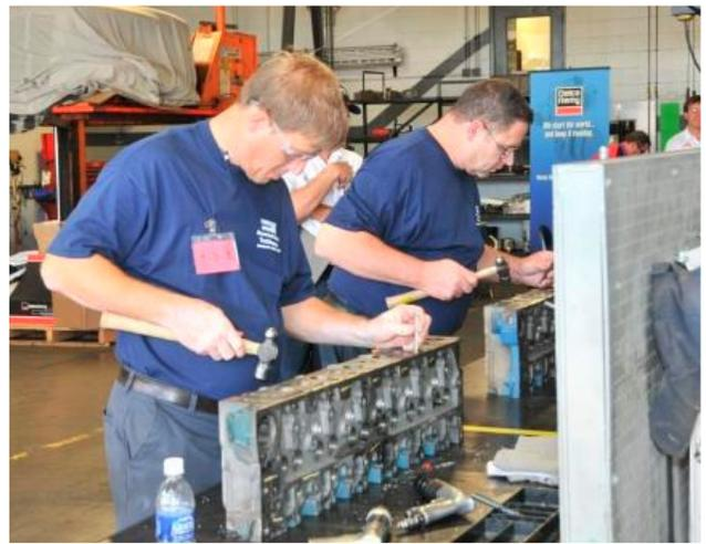
Two technicians work to complete a station involving a broken head bolt R&R
